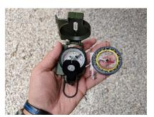
Military compass vs. a plastic-plate "orienteering" compass. More accurately referred to as a Lensatic Compass, a genuine military compass is exceptionally durable yet a precise instrument, designed to be used outdoors in any weather with a topographic map. As the term suggests, this type of compass has a lens which is used to read the compass dial and set a direction of travel.
